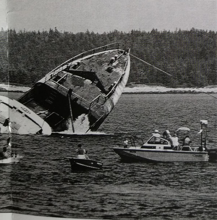
Photo below: Final sinking after approximately 2:30 hours of flooding
